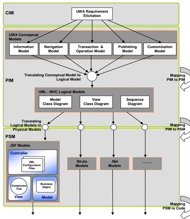
Fig. 3. An overview of the UWA-based MDD process.
