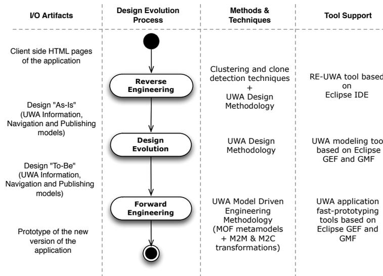
Fig. 3 The RE-UWA web application design evolution approach.
