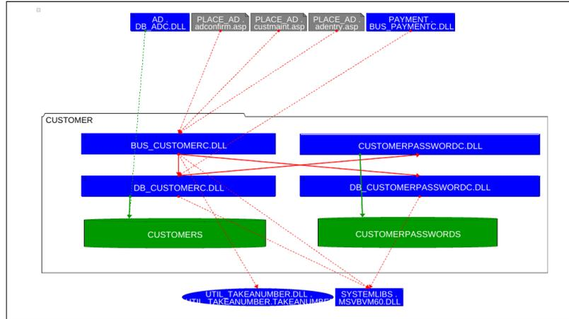
**Fig. 2** Architectural view of a web system's components: Blue boxes are DLL files, gray boxes are ASP files, blue ovals are COM objects, green tubes are databases [49].
